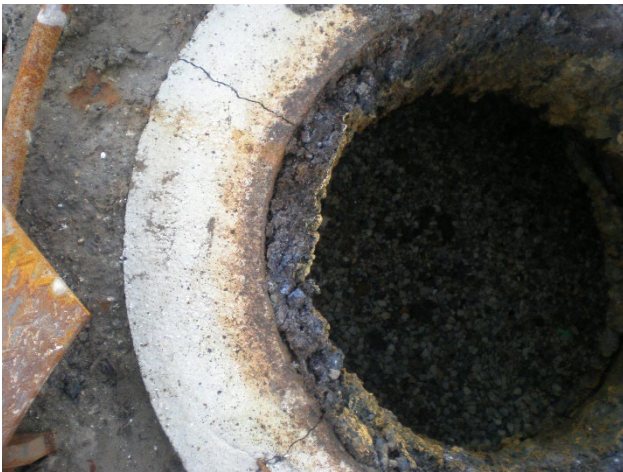
Figure 12. The photo above shows slag build up in the tapered electrode can.
