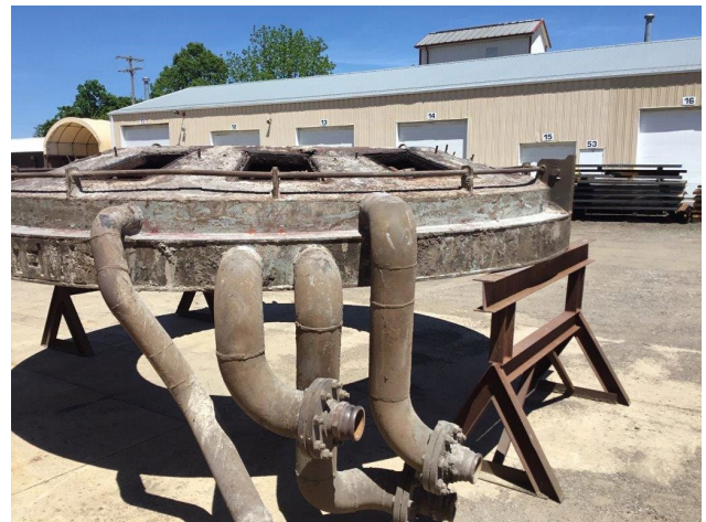
Figure 14. The photo above shows the returned spray-cooled damaged roof.
