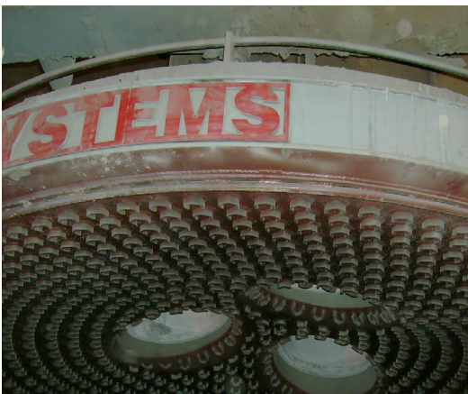
Figure 9. This photo shows the (3) electrode can openings and illustrates the slag retention system on the hot face.
