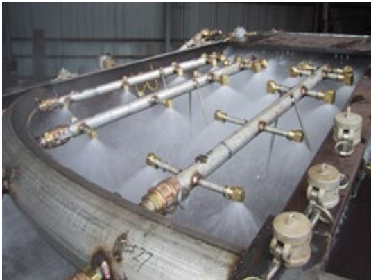
Figure 2. Spray water droplet impingement on the hot face plate.
