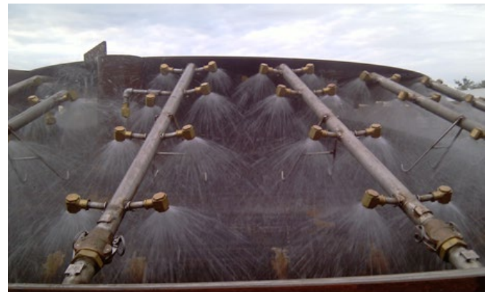
Figure 4. Removable spray bars and overlapping water sprays are shown. (The dust cover is not shown.)
