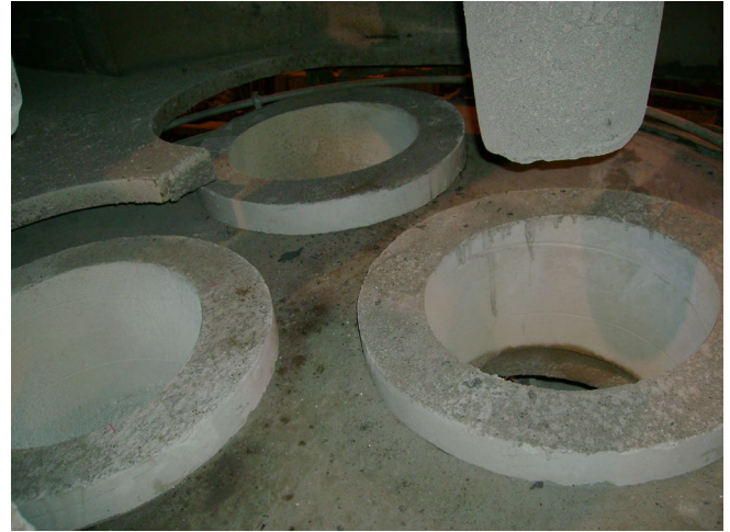
Figure 10. This photo shows the three refractory cans that insulate and protect the steel roof.
