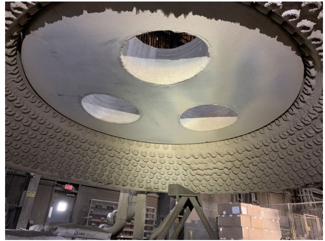
Figure 13. The new roof with new a 1-piece refractory delta replacement for the previous 3-piece delta.
