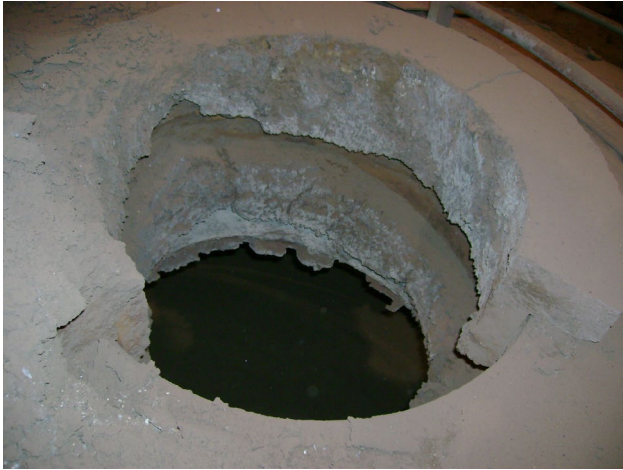
Figure 11. This photo shows the damaged refractory cans.
